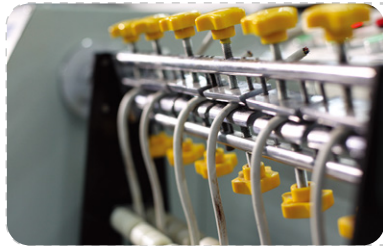
Bend-resistant cable, withstanding more than 400,000 tests
